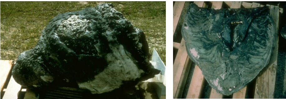
Figure 3. Vitrified soil column and cross section produced in the WSRC/GIT 1 MW scale test.
