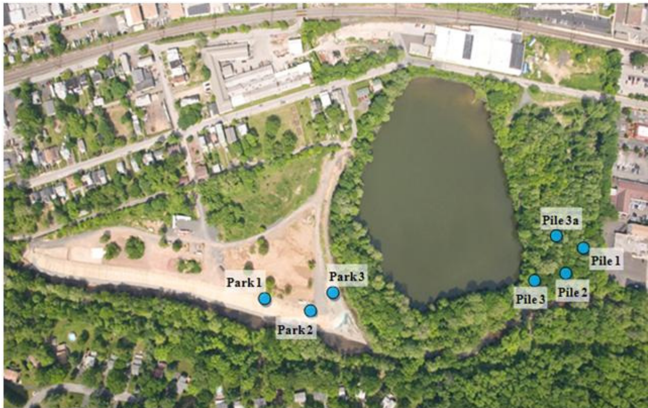
Figure 2- Map of approximate piezometer locations at the BoRit asbestos site
